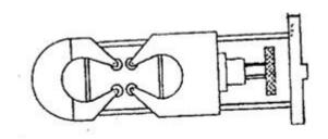
Fig.4-Tension Test Shackles
