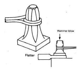
**Upsetting:** This is just opposite to drawing and involves increasing of the cross sectional area usually by pressing or hammering in the direction parallel to the original in got axis. Only the part to be upset is heated to forging temper and the bar or work is then struck at the end, usually between the hammer and the axis as shown in figure.
