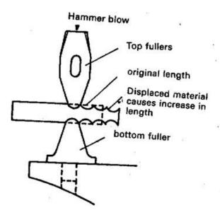
**Fullers:** are blunt hosed chisel and are used to reduce the thickness of hot metal. They may be held with hand fitted with a rod handle. Bottom fullers may be inserted in the square hole of the anvil.
