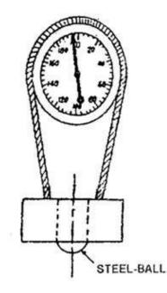
Mould hardness tester
