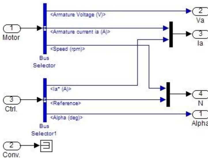
2. Connect the Motor, Conv., and Ctrl outputs of the DC3 block to the Motor, Conv., and Ctrl inputs of your Signal Selector block.
