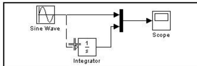
The software draws a line between the starting point and the input port of the Integrator block.
