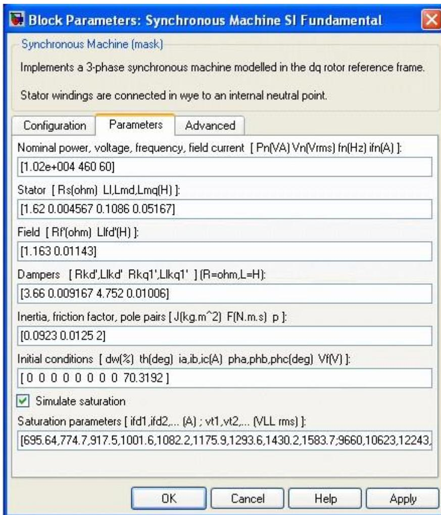
**Block Parameters: Synchronous Machine SI Fundamental**
