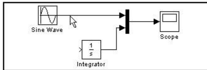
2. Press and hold the **Ctrl** key, then drag a line to the Integrator block's input port.
