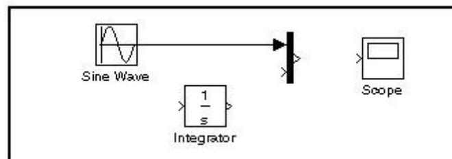
4. Drag a line from the output port of the Integrator block to the bottom input port on the Mux block.
