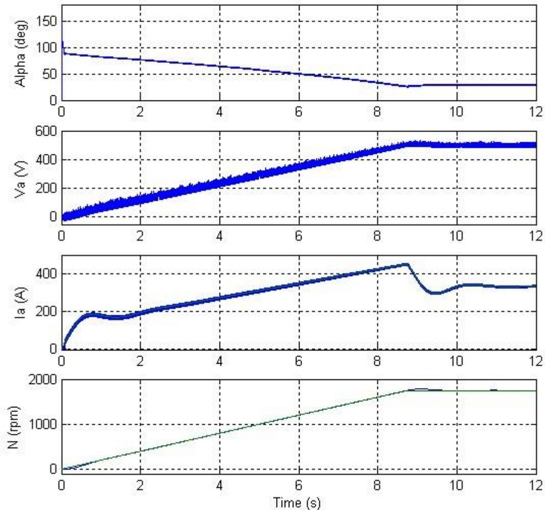
The current regulation is very good, and no current regulator changes will be undertaken. The speed regulation is satisfactory, but some improvements can be made: the initial tracking of the speed reference can be faster, and the speed overshoot and the small speed ramping error encountered during the accelerating phase can be reduced. A modification of the proportional and integral gains of the PI speed regulator allows you to achieve these goals:
