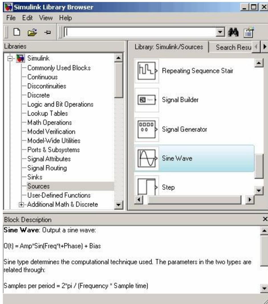
2. Select the Sine Wave block in the Simulink Library Browser, then drag it to the model window. A copy of the Sine Wave block appears in the model window.
