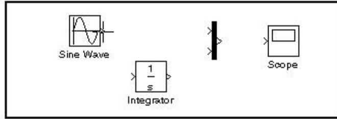
2. Drag a line from the output port to the top input port of the Mux block.
