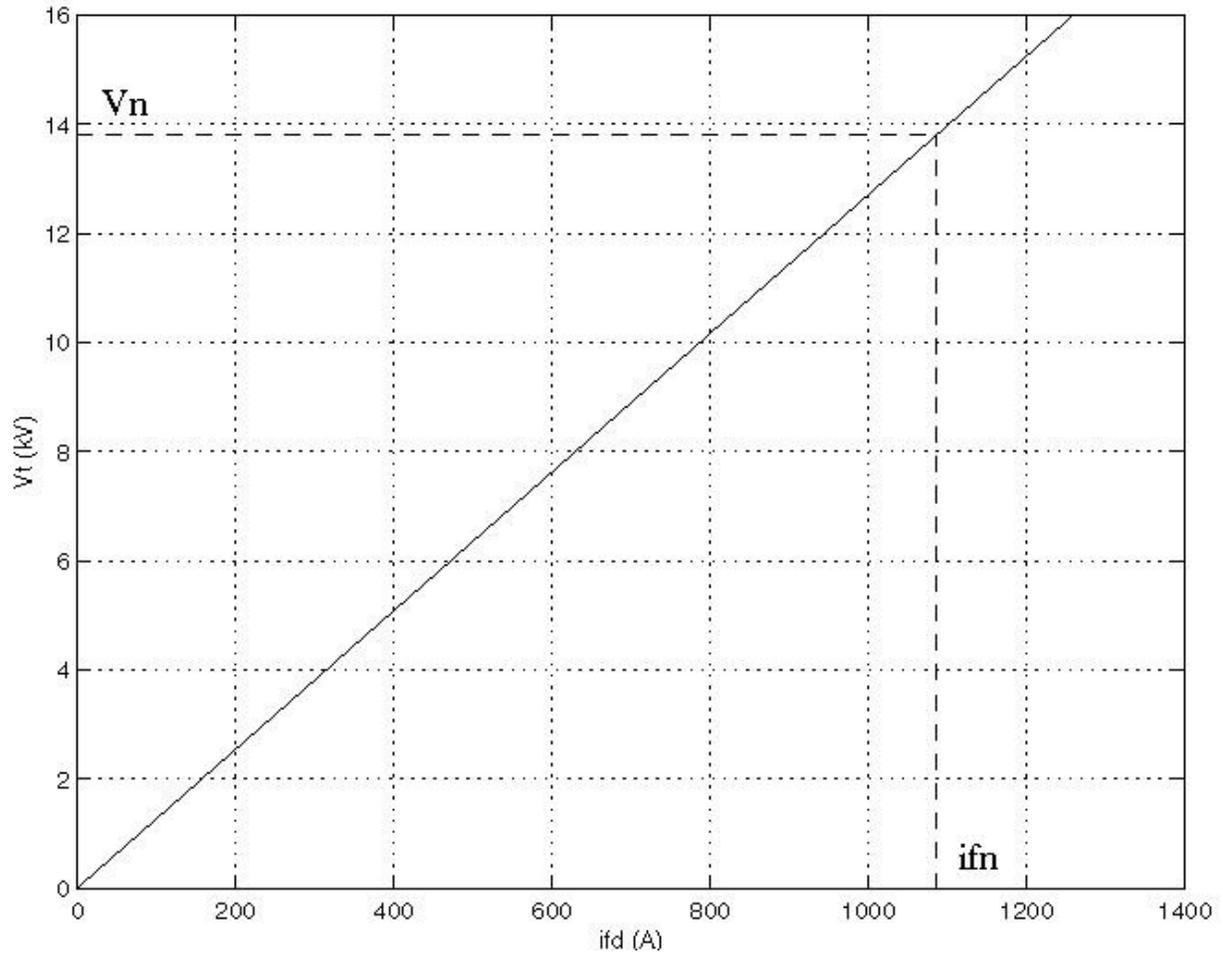
Saturation is modeled by fitting a polynomial to the curve corresponding to the matrix of points you enter. The more points you enter, the better the fit to the original curve.
