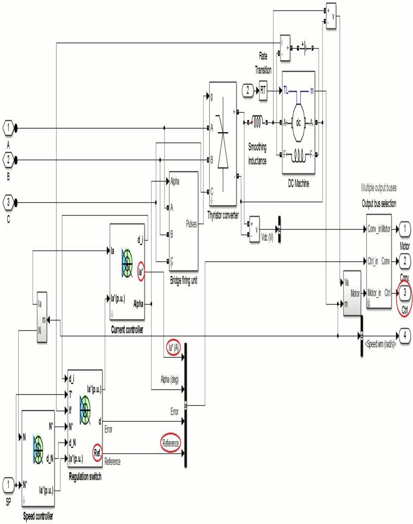
Internal bridge current and voltage signals can be extracted via the Conv. output, which is connected to a multimeter output. To view these signals, add a Multimeter block from the **Simscape > Electrical > Specialized Power Systems > Fundamental**
