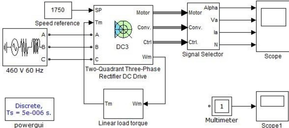
The example uses the DC3 model with a 200 hp DC motor parameter set during speed regulation. The DC3 block models a two-quadrant three-phase thyristor converter drive. The motor connects to a load and is driven to its 1750 rpm nominal speed.
