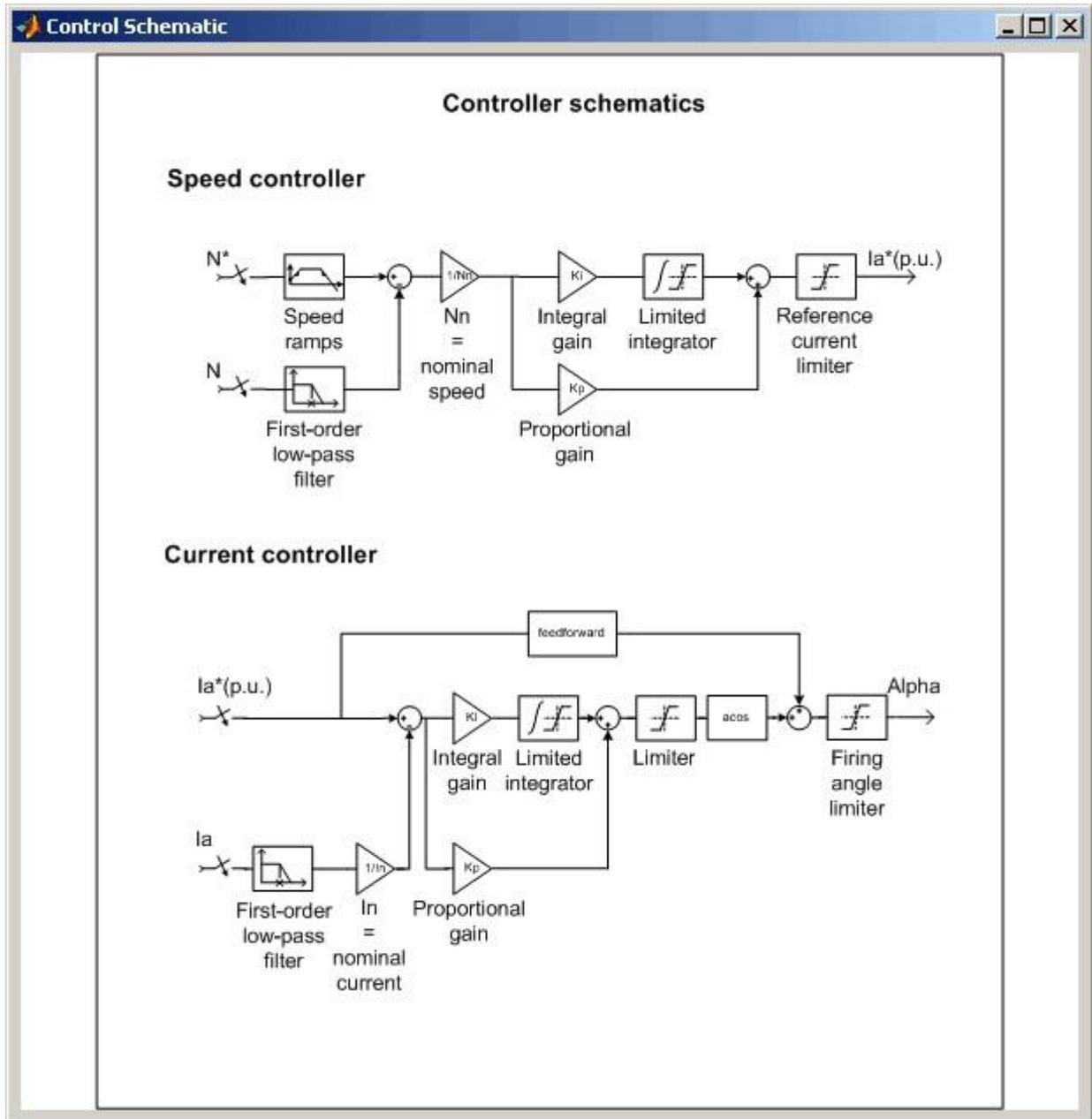
All default regulation parameters (speed and current controller parameters) have been trimmed for “no-load” inertias. Because the inertia has been modified, some changes need to be made in the speed controller. The current controller should not be modified, the change of inertia having little influence on the current control.
