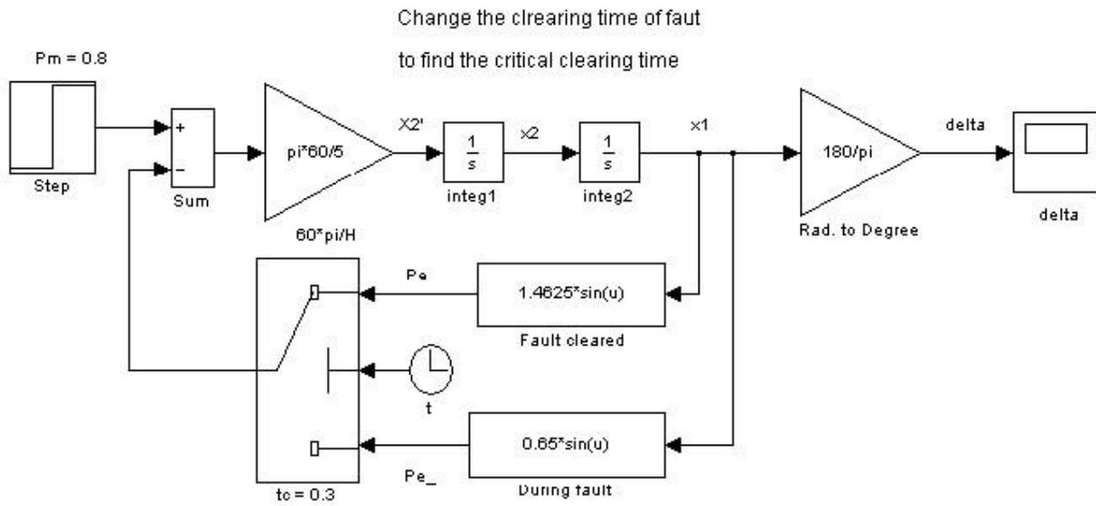
To change the clearing time of fault open the switch dialog box and change the Threshold setting.
