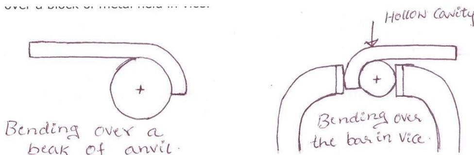
When the metal is bending by hammering, the outer and inner surface does not remain same. The inside surface is shortened while the outer surface is stretched which causes bulging of the side at the inner surface and a radius on the outer surface of a sharp corner is required an additional metal is required at the place where the bend occur in order to permit stretching of metal at outer surface.
