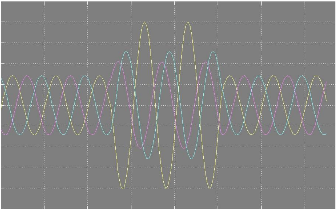
Fig: 1.5 – Current Waveform of Line – Ground Fault
